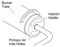
Figure 41 - Injector Holder On Outlet Burner Tube
